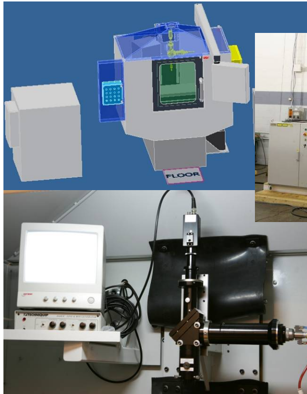
Close-Up of optics, prism targeting, camera and monitor
